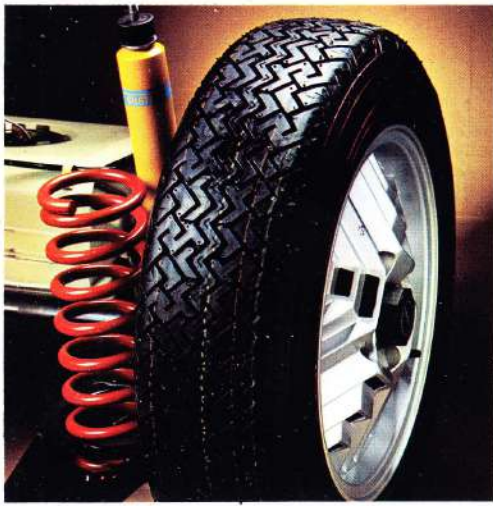
Coil springs combined with Bilstein gas shock absorbers all around to keep more tire on the road.
