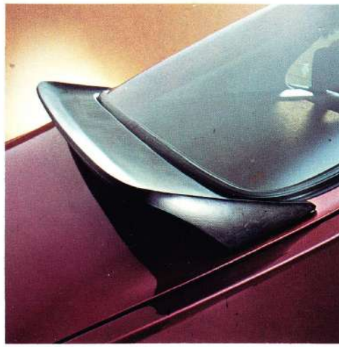
The rear spoiler improves stability and reduces fuel consumption at high speeds.
