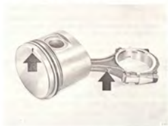
MOUNTING POSITION OF THE PISTON
