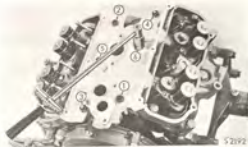
TIGHTENING SEQUENCE INDUCTION MANIFOLD BOLTS
