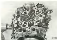
ASSEMBLED CYLINDER HEAD WITH MARKED SURFACES FOR APPLICATION OF SEALING COMPOUND
