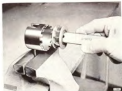
PLACING THE HUB IN THE TOOL Tool 87 90 305 (87 90 313 + 87 90 321)
