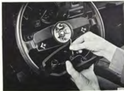
THE ELECTRIC CONNECTION IS REMOVED FROM THE HORN CONTACT
