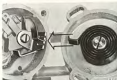
FITTING THERMOSTATIC SPRING
