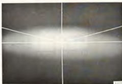
CORRECT LOW-BEAM SETTING FOR SEALED BEAM HEADLIGHT
