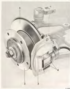
FRONT AXLE ASSEMBLY WITH DISC BRAKE
