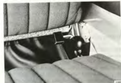
CATCH, AUXILIARY JUMP SEAT, SAAB 95 MODEL 1971-1975
