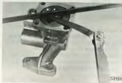
CHECKING AXIAL CLEARANCE OF ROTOR
