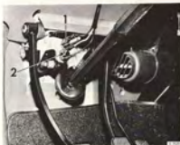
BRAKE WARNING SWITCH AND STOP LIGHT SWITCH
