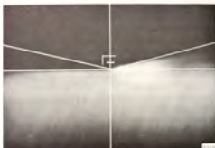
CORRECT SETTING FOR HEADLIGHTS, UP TO AND INCL. MODEL 1975 (RIGHT ASYMMETRIC LIGHT)
