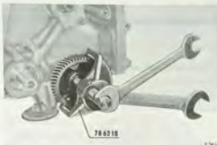
REMOVAL OF CRANKSHAFT GEAR Tool 78 62 188
