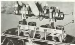
INSTALLATION OF ROCKER ASSEMBLY
