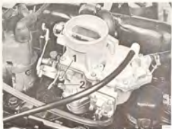
ADJUSTING THE IDLING SETTING
