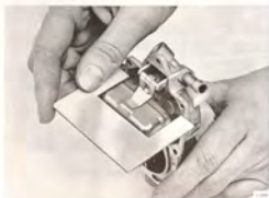
MEASURING THE FLOAT LEVEL WITH A GAUGE
