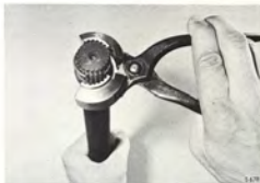
PLACING THE LOCK RING IN TOOL 78 41 612
