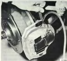
LOCATION OF BLEEDING NIPPLE, FRONT WHEEL BRAKE
