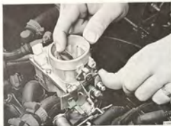
CHECKING FAST IDLING SETTING
