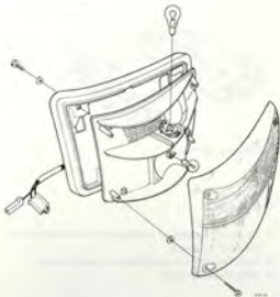
FLASHER AND PARKING LIGHT, FRONT, AS FROM MODEL 1978
