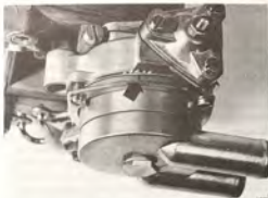
INSTALLATION MARK, AUTOMATIC CHOKE
