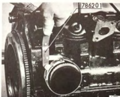
REMOVAL OF OIL FILTER CARTRIDGE
