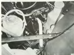
LEFT-HAND PIPE FIXED AGAINST THE ENGINE BLOCK
