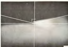
CORRECT SETTING FOR HEADLIGHTS, AS FROM MODEL 1976 (RIGHT ASYMMETRIC LIGHT)
