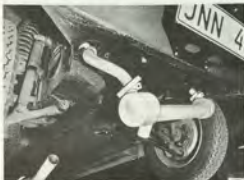
RIGHT-HAND PIPE IS WITHDRAWN THROUGH THE HOLE IN THE FLOOR
