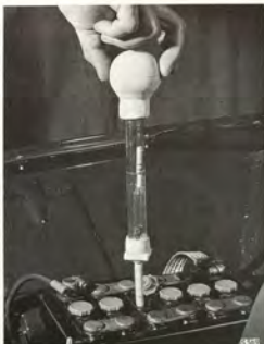
CHECKING THE BATTERY WITH A SYRINGE
