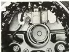
BRUSHES PUSHED UP AND SECURED
