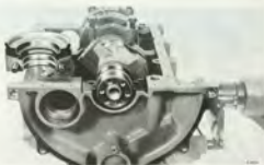
REAR BEARING CAPS WITH MARKED SURFACES FOR APPLICATION OF SEALING COMPOUND
