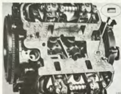
INSTALLATION OF INDUCTION MANIFOLD GASKET
