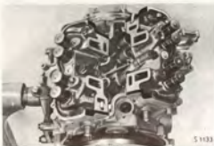
ASSEMBLED CYLINDER HEAD WITH MARKED SURFACES FOR APPLICATION OF SEALING COMPOUND
