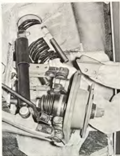
REMOVAL OF FRONT COIL SPRING Tool 78 40 820
