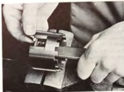
THE ROLLERS ARE INSTALLED Tool 87 90 305 (87 90 313 + 87 90 321)
