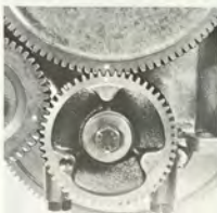
INSTALLATION MARKS, TRANSMISSION GEAR
