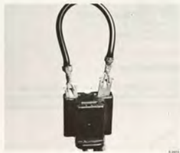
TERMINALS DF AND D+ CONNECTED
