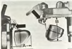
CHECK MEASUREMENT, FLOAT
