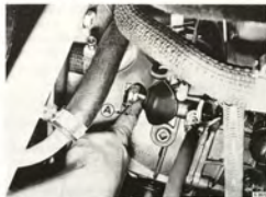
ADJUSTING THE CLUTCH CLEARANCE Correct clutch clearance: A = 0.16 in. (4 mm)
