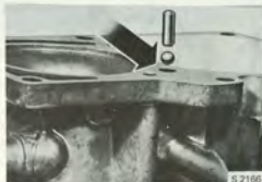
BALL AND WEIGHT, ACCELERATING PUMP FUEL CHANNEL
