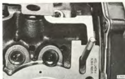
INSTALLATION OF CYLINDER HEAD GASKET
