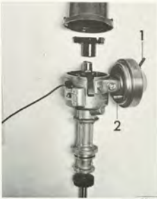
DISTRIBUTOR WITH DOUBLE ACTING VACUUM CONTROL UNIT
