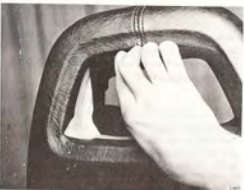
THREADING THE PLASTIC RING OUT FORWARDS
