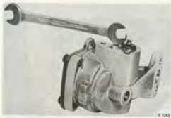
REMOVAL OF RELIEF VALVE COVER PLATE
