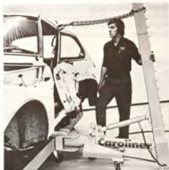
EXTENSION PIECE MOUNTED TO DRAW-ALIGNER ARM FOR THE APPLICATION OF LOADS AT ROOF HEIGHT
