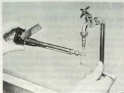
THE FLAP VALVE HAS MOVED TO ITS LEFT POSITION
