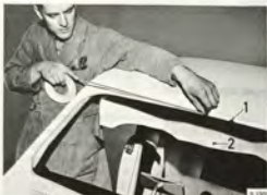
FITTING DOUBLE ADHESIVE TAPE
