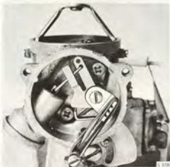
THE THERMOSTATIC SPRING HAS BEEN REPLACED BY A RUBBER BAND
