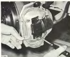
INSTALLATION OF BRAKE PADS
