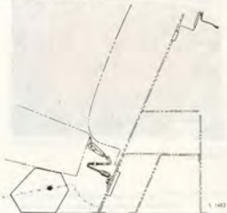
LOCKING DEVICE FOR CUSHIONS, REAR SEAT, SAAB 96
