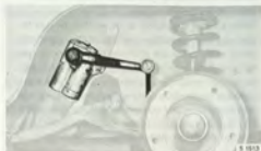
REAR SHOCK ABSORBER, SAAB 95
