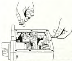
COLLECTING TOOL 78 40 697 WHEN SHIFT FORK RAIL HAS BEEN DRIVEN IN
