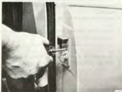
ADJUSTMENT OF DOOR STRIKER PLATE
