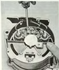
DISCONNECTING THE BRUSH UNIT ASSEMBLY WIRE
