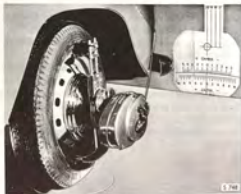
WHEEL ALIGNMENT WITH OPTICAL MEASURING EQUIPMENT
