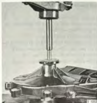
REMOVAL OF FAN BEARING Tool 78 62 436 and drift
