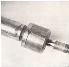
SECURING LOCK PIN WITH CENTER PUNCHES
