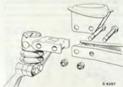
REMOVAL OF UPPER BALL JOINT AND LOWER SPRING SEAT
