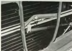
CENTRAL BUSHING FIXED WITH TENSION PIN, MODEL 1973
