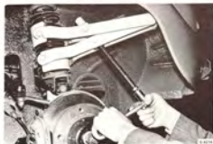
THE POSITION OF THE SPRING SCISSORS AND THE SPRING CUPS ON THE RIGHT SIDE
