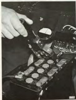
CHECKING THE BATTERY WITH A CELL TESTER
