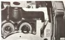
INSTALLATION OF CYLINDER HEAD GASKET
