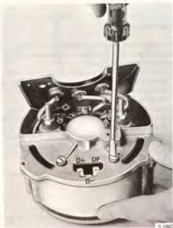
UNSCREWING THE BRUSH UNIT ASSEMBLY
