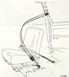
SEAT BELT, 3-POINT TYPE, AS FROM MODEL 1968 UP TO AND INCL. MODEL 1973
