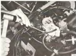
FITTING A NEW PLASTIC PLUG
