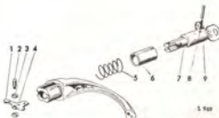
OUTER HANDLE, UP TO AND INCL. MODEL 1971
