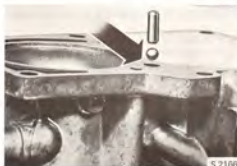
BALL AND WEIGHT, ACCELERATING PUMP FUEL CHANNEL
