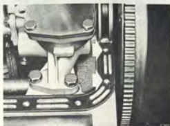
FITTING THE TWO BOLTS WITH RUBBER WASHERS
