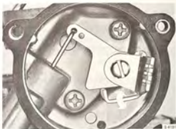
ADJUSTMENT OF THERMOSTATIC SPRING LEVER TONGUE
