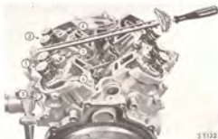
TORQUING THE CYLINDER HEAD
