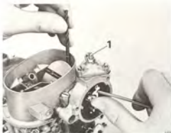
CHECKING THE VACUUM CONTROL, CHOKE VALVE 1. Adjustment screw
