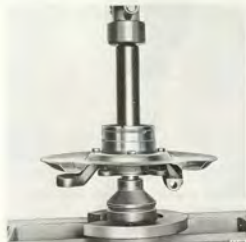
PRESSING THE KNUCKLE HOUSING AND BEARING ONTO THE OUTER DRIVE SHAFT Tool 78 41 067
