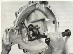
REMOVAL OF THE SEALING RING FROM THE CLUTCH SHAFT
