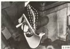
ADJUSTMENT OF LINK ROD
