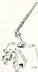
GEAR SHIFT SHAFT UNIVERSAL JOINT, R.H.D. DRIVE CAR
