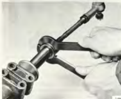
REMOVAL OF OUTER BEARING CUP AND LOCK NUT Tools 78 40 713 and 78 39 624
