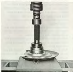
PRESSING IN THE BALL BEARING IN THE STEERING KNUCKLE HOUSING Tools 78 40 754 and 78 40 309
