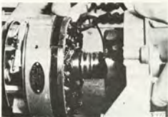
REMOVAL OF DRIVE END PLATE AND ROTOR
