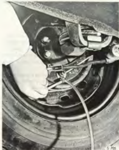
LOCATION OF BLEEDING NIPPLES, REAR WHEEL BRAKE
