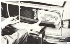
REMOVING THE PROTECTIVE PLATE, AS FROM MODEL 1974
