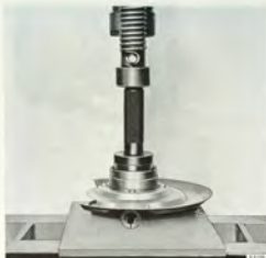
PRESSING IN THE BALL BEARING IN THE STEERING KNUCKLE. THE MARK ON THE BALL BEARING FACING OUTWARDS.
