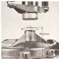
INSTALLATION POSITION FOR FAN PULLEY FLANGE
