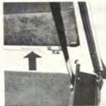
Chassis number imprinted in car body
