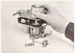
THE FLOAT CHAMBER COVER IS LIFTED OFF
