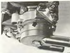
INSTALLATION MARK, AUTOMATIC CHOKE
