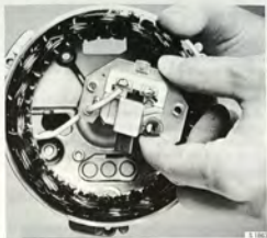
REMOVING THE BRUSH UNIT ASSEMBLY
