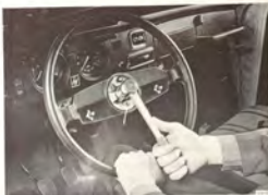
REMOVING THE STEERING WHEEL NUT
