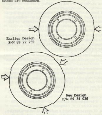
LOOSE STEERING WHEEL SHAFT FIX
