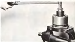
TIGHTENING THE PINION NUT Fixture 8790636 with retainer ring
