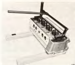
REMOVING THE VALVES Tool 8392300
