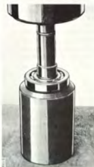
EXPELLING THE SHAFT FROM THE BEARING Tool 8390536
