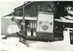
MEASURING THE VOLTAGE ACROSS TERMINALS 30 (+) AND 87 (-) IN THE RELAY HOLDER
