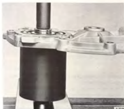
PRESSING OUT THE GEAR Drift 8390189, support 8390098
