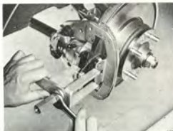
REMOVAL OF BRAKE PADS WITH EXTRACTOR 8995771
