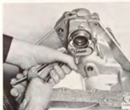
REMOVING THE SEALING RING, MODEL 1976-1977
