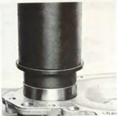
PRESSING IN THE GEAR AND BALL BEARING IN THE BEARING HOUSING Sleeve 8390098 and ring 8390247
