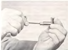
LOCKING THE RATCHET SLEEVE, VERSION A
