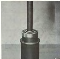
PRESSING THE BEARING OFF THE INPUT GEAR Drift 8390189, supports 8390098 and 8390247
