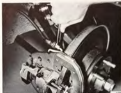
DISCONNECTING THE BRAKE PIPE
