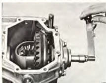
MEASURING THE DIFFERENTIAL BEARING TORQUE Torque wrench and driver 8790818
