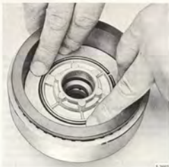
INSERTING PISTON IN FRONT CLUTCH Tool 8790107
