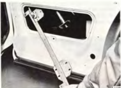
REMOVING THE REAR-DOOR WINDOW REGULATOR
