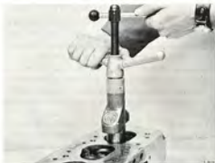
INSTALLING THE VALVE GUIDE Tool 8390437
