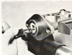
REMOVING THE CIRCLIP ON THE PRIMARY PISTON
