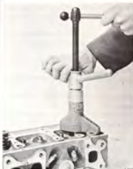
REMOVING THE VALVE GUIDE Tool 8390437
