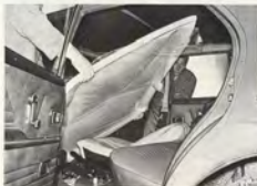
THE LINING IS MOVED IN, 4-DOOR MODEL
