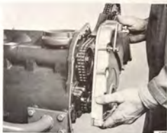
REMOVING THE CHAIN TRANSMISSION COVER
