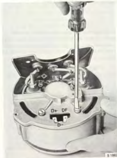
UNSCREWING THE BRUSH UNIT ASSEMBLY
