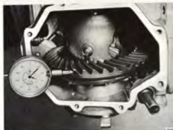
MEASURING GEAR BACKLASH, MANUAL TRANSMISSION
