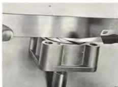
CHECKING THE AXIAL CLEARANCE
