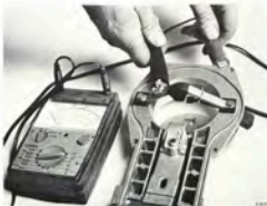
CHECKING THE STOP BRACKET INSULATION, UP TO AND INCL. MODEL 1976
