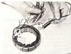
MEASUREMENT OF RESISTANCE ACROSS TWO PHASES (V-W)
