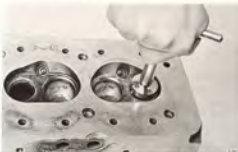
MILLING VALVE SEATS Tool 8392193
