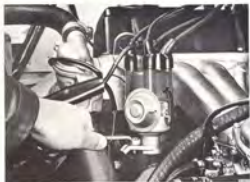
REMOVING DISTRIBUTOR, AS FROM MODEL 1977
