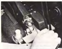
ADJUSTING THE HANDBRAKE CABLE
