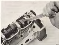
TURNING THE CAMSHAFT ON A REMOVED CYLINDER HEAD
