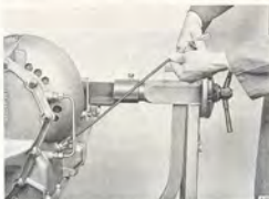
CLAMPING THE STOP CLIP ONTO THE THROTTLE CABLE
