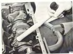
REMOVING PISTON AND CONNECTING ROD
