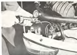
VACUUM PUMP AND GAUGE CONNECTED TO THE WHITE CONNECTION
