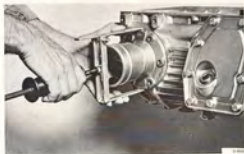
REMOVING THE DIFFERENTIAL BEARING CAP Tool 8790776 and 8390270
