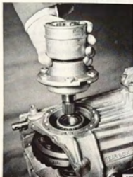
DIFFERENTIAL BEARING CAP WITH INNER DRIVER
