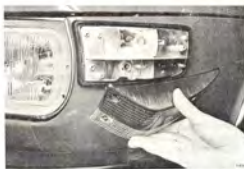
CHANGING BULBS, FRONT, UP TO AND INCL. MODEL 1976
