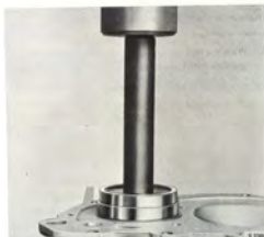
PRESSING OUT THE BEARING FROM THE BEARING HOUSING Drift 8390189, sleeve 8790460
