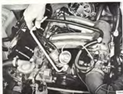
REMOVING DISTRIBUTOR RETAINING SCREWS, UP TO AND INCL. MODEL 1976
