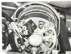
ALTERNATOR WIRING CONNECTIONS AND COLOR CODE, MAKE SEV
