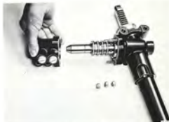
FITTING THE VALVE HOUSING. THE VALVE SHAFT IS FITTED WITH FITTING CONE 8995979
