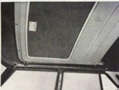
REMOVING THE SUNROOF FRAME
