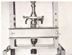
PRESSING ON THE INNER RACE OF THE BEARING
