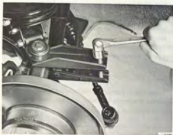
REMOVING THE UPPER BALL JOINT Tool 8995409
