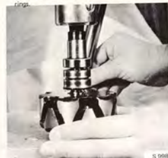
PRESSING THE BALL BEARING INTO PLACE ON THE SLIP RING SIDE
