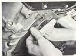
FITTING THE EXHAUST MANIFOLD GASKETS (AS FROM MODEL 1976)
