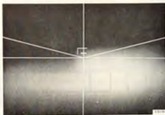
CORRECT LOW-BEAM SETTING FOR SEALED BEAM HEADLIGHT
