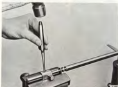
REMOVING THE COTTER PIN FROM THE DRIVER
