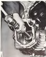
MOUNTING THE PINION SHAFT
