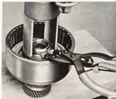
REMOVING LOCK RING FOR RETURN SPRING IN REAR CLUTCH
