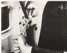
ADJUSTING VERTICAL AND FRONT- AND-REAR FIT OF FRONT DOOR
