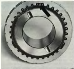
POSITIONING OF A SPRING END IN THE SPACE BETWEEN THE TEETH OF THE RING
