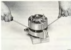
SEPARATING THE STATOR AND SLIP RING CAP FROM THE DRIVE BEARING CAP AND ROTOR
