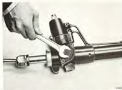
ADJUSTING THE RADIAL PLAY OF THE RACK
