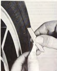
FITTING WEIGHTS TO ALUMINIUM WHEELS
