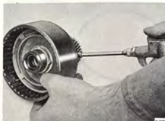
REMOVING REAR CLUTCH PISTON WITH THE AID OF COMPRESSED AIR
