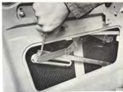
FREEING THE PLASTIC RUNNER FROM THE GUIDE SLOT
