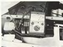
MEASURING THE VOLTAGE ACROSS TERMINALS 86 (+) AND 85 (-) IN THE RELAY HOLDER
