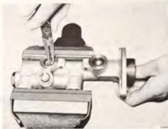
REMOVING THE STOP PIN ON THE SECONDARY PISTON
