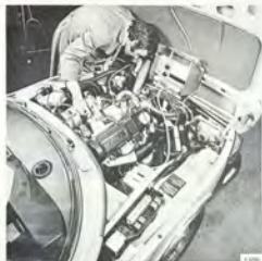
IGNITION SETTING WITH STROBOSCOPE LAMP
