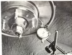
MEASURING THE BRAKE DISC THROW
