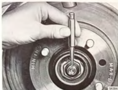
UPSETTING THE FLANGE OF THE LOCKING NUT
