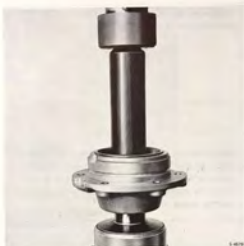
MOUNTING THE CAP IN A PRESS Tool 7841067
