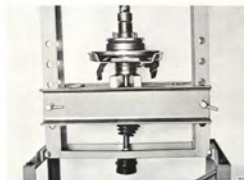
PRESSING THE WHEEL HUB ONTO THE SHAFT
