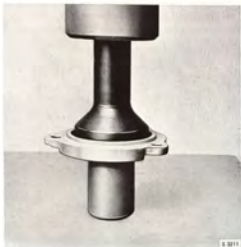
INSTALLING THE SEALING RING IN THE GUIDE SLEEVE Model 1975, drift 83 90 320
