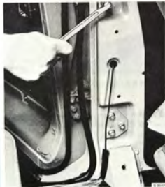
REMOVING REAR DOOR, 4-DOOR MODEL
