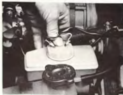
CHECKING THE LEVEL WARNING SYSTEM
