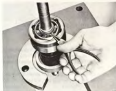
OPENING THE CIRCLIP WITH CIRCLIP PLIERS
