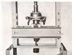
FITTING THE HUB AND BRAKE DISC TO THE SHAFT
