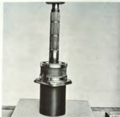
PRESSING THE SHAFT OUT OF THE BEARING HOUSING Sleeve 8390098
