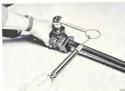
CHECKING THE STEERING GEAR TORQUE Tool 8995607 and dynamometer
