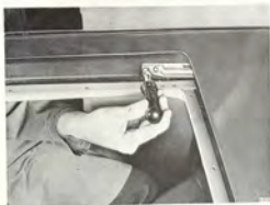
THE TWO SCREWS IN THE FRONT ENDS OF THE GUIDE RAILS ARE INSTALLED
