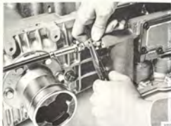
REMOVING THE GEAR SELECTOR LEVER CABLE Tool 8790388
