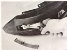
FITTING THE BRACING STRIP, UP TO AND INCL. MODEL 1976
