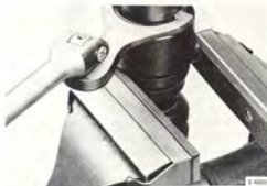
REMOVING THE RING NUT Tool 8995961
