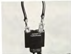
TERMINALS DF AND D+ CONNECTED
