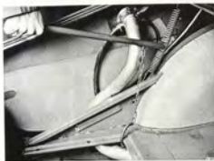
REMOVAL OF SPRING, TRUNK LID Tool 8291577
