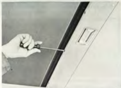
REMOVAL OF THE FOUR SCREWS IN THE FRONT EDGE
