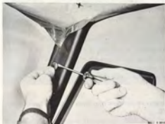
REMOVING THE FRONT PILLAR SAFETY PADS
