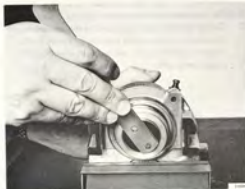
BRAKE HOUSING WITH PISTONS Tool 8996043
