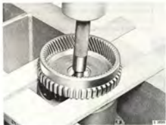
SEPARATION OF RING GEAR AND PINION UNDER PRESSURE Drift: 8790610
