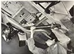
REMOVING THE STEERING GEAR FROM THE CAR
