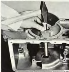
REMOVING THE BEARING IN THE TORQUE CONVERTER HOUSING
