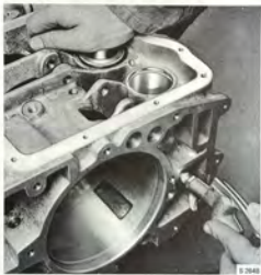
REMOVING THE REAR PISTON
