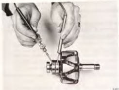
MEASURING THE RESISTANCE OF THE ROTOR WINDING
