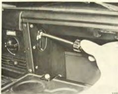
REMOVING THE TIDY BOX
