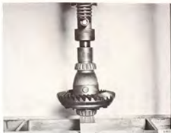
PRESSING ON THE DIFFERENTIAL JOURNAL BEARINGS Tool 8790487
