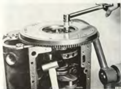
TIGHTEN THE FLYWHEEL SCREWS TO SPECIFIED TORQUE
