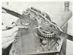
CHECKING ALIGNMENT OF CRANKSHAFT SPROCKET
