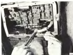
THE PIPE CONNECTIONS ARE CHECKED WITH THE AID OF A MIRROR
