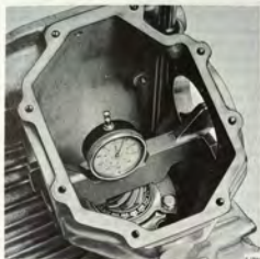
MEASURING TOOL LOCATED IN DIFFERENTIAL BEARING OPENINGS, MANUAL TRANSMISSION
