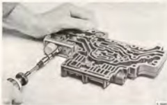
REMOVING THE END PLATE
