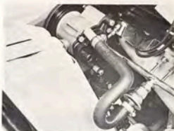
AIR INJECTION SYSTEM: THE HOSE TO THE CHECK VALVE REMOVED AND PLUGGED
