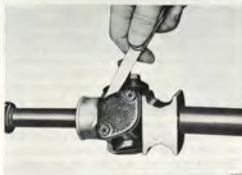
MEASURING CLEARANCE BETWEEN CAP AND HOUSING
