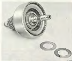
REAR CLUTCH HUB WITH WASHERS
