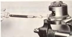
CHECKING PRE-LOAD WITH SPRING BALANCE Fixture 8790636 with retainer ring
