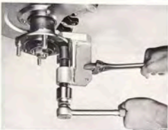
INSTALLING A WHEEL BOLT Tool 8995920
