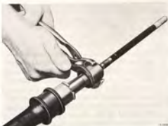
REMOVING OUTER BEARING CUP AND LOCK NUT Tool 8390197 and polygrip pliers
