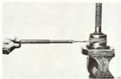
CHECKING THE BEARING HOUSING TORQUE Fixture 8790636, holder ring 8790651 and dynamometer
