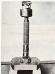
PRESSING THE REAR BEARING OFF THE SHAFT Fixture 8790636 and holder ring 8790651
