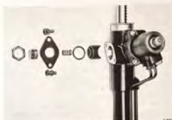
RADIAL ADJUSTMENT OF THE RACK
