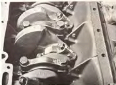
MARKS ON CONNECTING RODS, MAIN BEARINGS AND CYLINDER BLOCK
