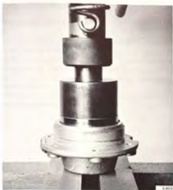
PRESSING IN THE BEARING TRACKS Tool 8390114
