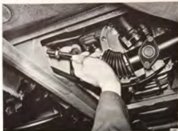
BEND THE LEFT TIE ROD DOWN THROUGH THE OPENING IN THE BODY
