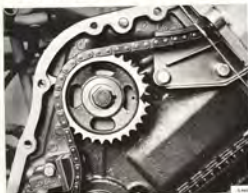
IDLER SHAFT MARKING. THE BULGE IN THE HOLE ON THE IDLER SHAFT CHAINWHEEL SHOULD LINE UP WITH THE SMALL HOLE IN THE KEEPER PLATE.
