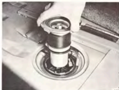
LIFTING OUT THE FUEL PUMP
