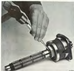
LOCKING THE PINION BEARING NUT
