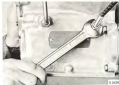
REMOVING THROTTLE CABLE FROM TRANSMISSION CASING
