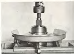
THE OUTER DRIVE SHAFT IS PRESSED OUT
