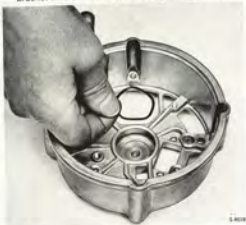
PLACING THE SNAP RING IN THE SLIP RING END BRACKET
