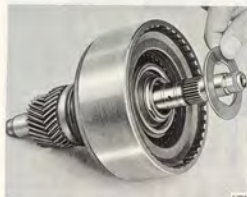
LOCATION OF THE WASHER ON REAR CLUTCH HUB
