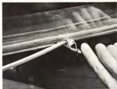
APPLYING THE WINDSHIELD MOULDING Tool 8291023
