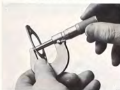
MEASURING GASKET AND SHIMS
