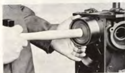
INSTALLING PISTON AND CONNECTING ROD Tool 7862287
