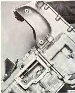
REMOVING TORQUE CONVERTER HOUSING
