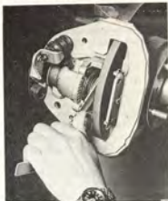
SCREWING THE BRAKE PISTON INTO THE FRONT BRAKE HOUSING WITH TOOL 8996043
