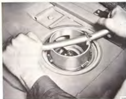
TURNING THE FUEL PUMP Tool 8392433
