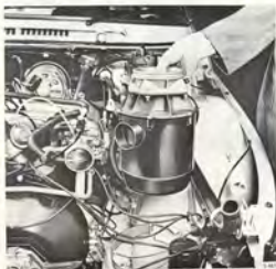
REMOVING THE AIR CLEANER AND MIXTURE CONTROL UNIT
