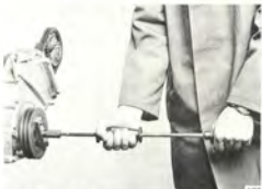
REMOVING THE BELT PULLEY Tools 8390270 and 8392151
