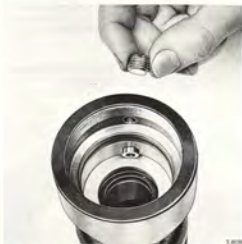
LOCKING THE CONE IN PLACE WITH A SPECIAL SCREW TOOL 8995953
