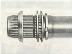
DRIVE SHAFT WITH LOCK RING AND WASHERS
