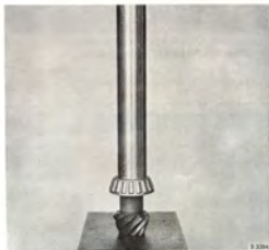
PRESSING ON THE ROLLER BEARING NEAREST THE PINION GEAR Sleeve 8390148
