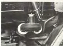
PULSE AIR SYSTEM: THE HOSE TO THE CHECK VALVES REMOVED AND PLUGGED
