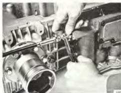
REMOVING THE GEAR SELECTOR WIRE Tool 8790388
