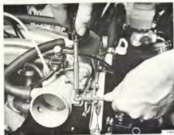
ADJUSTING THE THROTTLE VALVE STOP
