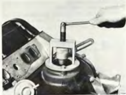
PRESSING IN THE PUMP SHAFT AND BEARING Tool 8392490 (or 8392649 and 8390551)
