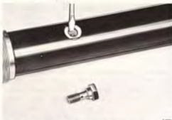
TURN UP THE HOLE IN THE KNURLED SLEEVE
