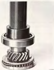
THE BALL BEARING IS PRESSED ONTO THE INPUT SHAFT Tools 83 90 148 and 87 90 867
