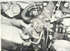
ADJUSTING THE DECELERATION VALVE Tool 8392466 and screw driver
