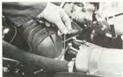
ADJUSTING THE CO-SETTING
