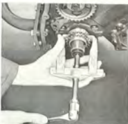
REMOVING THE CRANKSHAFT SPROCKET Universal puller and tool 8391849
