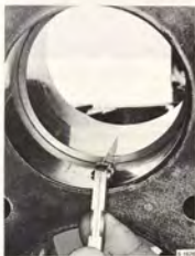
MEASURING PISTON RING GAP
