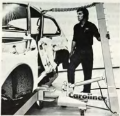
EXTENSION PIECE MOUNTED TO DRAW-ALIGNER ARM FOR THE APPLICATION OF LOADS AT ROOF HEIGHT
