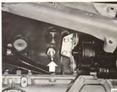
ENGINE BLOCK DRAIN COCK (SUPERSEDED BY A DRAIN PLUG ON LATER CARS OF MODEL 1977)
