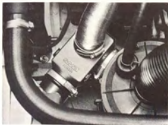
THERMOSTATICALLY CONTROLLED AIR PREHEATING, AS FROM MODEL 1978
