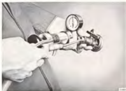
BLOWING THROUGH THE EGR VALVE
