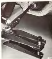
REMOVING THE STEERING ARM Tool 8995409
