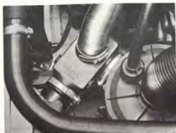
THERMOSTATICALLY CONTROLLED AIR PREHEATING, AS FROM MODEL 1978
