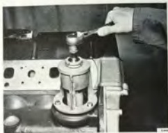
PRESSING IN THE BEARING HOUSING, VERSION II Tool 8392490
