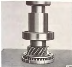
MOUNTING THE BEARING ON THE INPUT GEAR Sleeve 8790487
