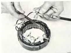
TEST OF STATOR WINDING
