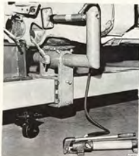
SIDE MOUNTING FOR USE WITH A 4-TON HYDRAULIC CYLINDER
