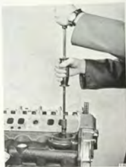
REMOVING THE WATER PUMP, VERSION I Tools 8390270 and 8392136
