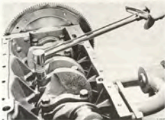
TIGHTEN THE MAIN BEARING SCREWS
