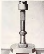
PRESSING OFF THE REAR PINION BEARING
