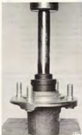
PRESSING IN THE BEARING OUTER RINGS
