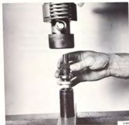
PRESSING THE BALL BEARING ONTO THE SHAFT
