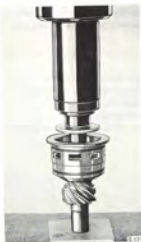
FITTING THE THROWER, VERSION I Tools 8390551 and 8390569
