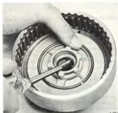
REMOVING FRONT CLUTCH PISTON WITH THE AID OF COMPRESSED AIR
