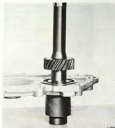
FITTING THE OUTPUT GEAR INTO THE BEARING HOUSING
