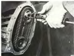
REMOVING THE SPROCKET WHEEL Tool 83 90 270 and 87 90 834
