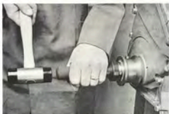
REMOVING THE CLUTCH SHAFT BEARING
