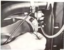
CHECKING RADIATOR FAN OPERATION, UP TO AND INCL. MODEL 1976
