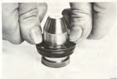
SLIDE THE SERVO SEAL ONTO THE FITTING SLEEVE USING THE FITTING CONE (SPECIAL TOOLS 8995938 AND 8995946)
