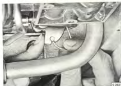
REMOVING THE THROTTLE CABLE FROM VALVE HOUSING
