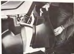
REMOVING THE SIDE TRIM BY THE REAR SEAT, 4-DOOR SAAB 99 WAGONBACK
