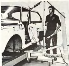
LOADS MAY BE APPLIED IN AN UPWARD DIRECTION BY MEANS OF AN ADDITIONAL HYDRAULIC CYLINDER AND AN EXTENSION PIECE
