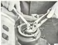
REMOVING THE IMPELLER CENTER SCREW
