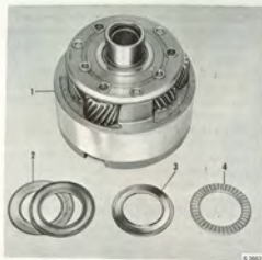
PLANET GEAR CARRIER WITH SHIMS AND THRUST NEEDLE BEARING
