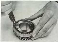
REMOVING THE SYNCHRONIZING RING FOR 3RD GEAR
