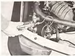
MEASURING THE SIGNAL FROM THE VACUUM SIGNAL SWITCH
