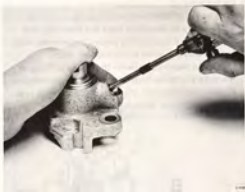
FORCING OUT THE INDIRECT PISTON WITH COMPRESSED AIR
