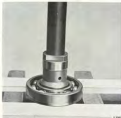
REMOVING THE BEARING FROM THE INPUT GEAR Drift 8390189, ring 8390213
