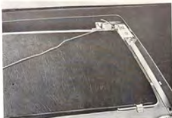
THE SPRINGS FOR THE COVER PLATE TENSIONED WITH BLOCKS EQUIPPED WITH STRINGS
