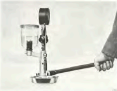
CLEANING BY MEANS OF INJECTOR TESTER
