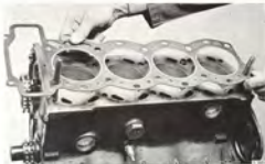
FITTING THE CYLINDER HEAD GASKET Tool 8392128
