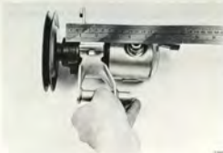
MOUNTING POSITION FOR PUMP IN LINE WITH DELIVERY LINE CONNECTION
