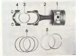
PISTON AND CONNECTING ROD WITH BEARINGS AND PISTON RINGS
