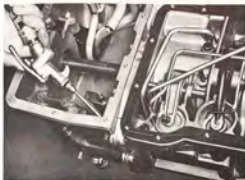
CHECKING THE AUTOMATIC ADJUSTMENT BY FORCING COMPRESSED AIR THROUGH THE HOLE FOR APPLYING THE SERVO
