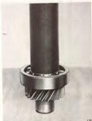
PRESSING ON THE BALL BEARING Sleeve 8390148
