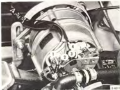
ALTERNATOR WIRING CONNECTIONS AND COLOR CODE, MAKE BOSCH
