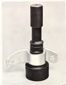
INSERTING A ONE-PIECE RUBBER BUSHING Tool 7841331
