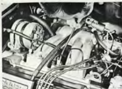
CHECKING THE PVS VALVE
