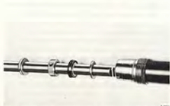
PUSH THE RACK WITH WASHER, SERVO SEAL, SLEEVE AND PLUNGER SEALS INTO THE SERVO CYLINDER
