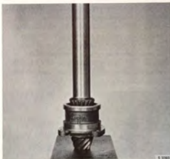
PRESSING IN THE FRONT ROLLER BEARING Sleeve 8390148
