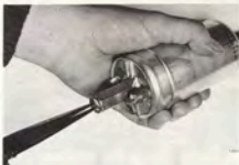
UNSCREWING THE NONRETURN VALVE, AS FROM MODEL 1978
