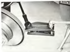
DISCONNECTING THE STEERING ARM FROM THE TIE ROD Tool 8995409
