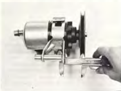
DISTANCE BETWEEN PUMP MOUNTING AND PULLEY CENTRE
