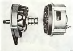
STATOR AND SLIP RING END BRACKET SEPARATED FROM ROTOR AND DRIVE BEARING ASSEMBLY
