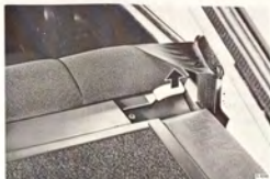
BACKREST CUSHION CATCH, SAAB 99 WAGONBACK, UP TO AND INCL. MODEL 1976
