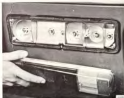
CHANGING BULBS, REAR, SAAB 99 L 199 GLJ AND 99 EMS, UP TO AND INCL. MODEL 1976
