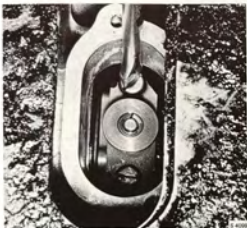
THE GOVERNOR SCREWS ARE REMOVED
