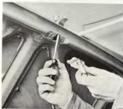
REMOVING THE LOCK FROM THE TRUNK LID
