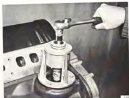
REMOVING THE WATER PUMP, VERSION II AND III Tool 8392490
