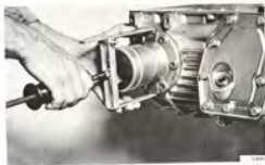
REMOVING THE DIFFERENTIAL BEARING SEATS Tool 8390270 and 8790776
