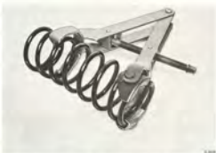
TOOL 8995839 APPLIED ON THE COIL SPRING
