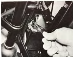
CONTROL WIRE LOOSENED FROM ACCELERATOR PEDAL
