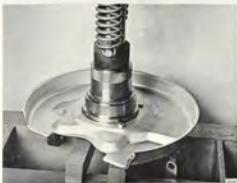
FITTING THE FRONT WHEEL BEARING Drift 8996068
