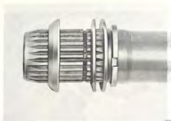
SHAFT WITH LOCK RING AND WASHERS
