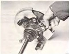
FITTING THE OUTER BELLOWS CLAMP Pliers 7844699
