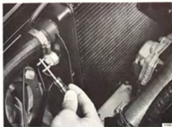
CHECKING RADIATOR FAN OPERATION, AS FROM MODEL 1977
