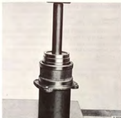
INSTALLING THE BEARING RACE IN BEARING HOUSING Drift 8390189, sleeve 8790461
