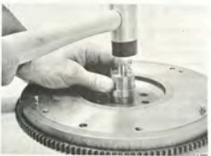
FITTING THE CLUTCH SHAFT BEARING
