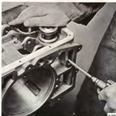
REMOVING THE FRONT PISTON
