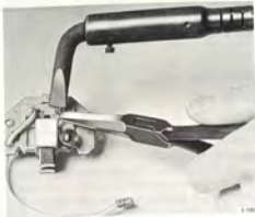
UNSOLDERING THE BRUSH UNIT TERMINALS
