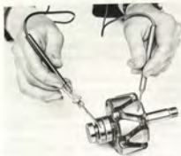
CHECKING THE INSULATION OF THE EXCITER WINDING AND THE SLIP RINGS
