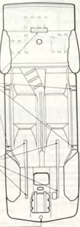
1:2 Entire underbody + wheel housing is sprayed with oil
