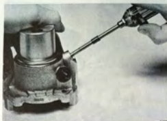
FORCING OUT THE INDIRECT PISTON WITH COMPRESSED AIR
