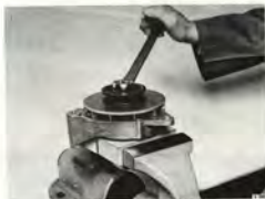
UNSCREWING THE PULLEY NUT; THE ROTOR IS HELD FAST BY TOOL 8580029
