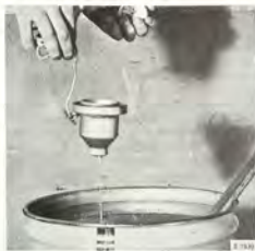
MEASURING VISCOSITY WITH AN SIS BEAKER
