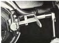
REMOVAL OF BRAKE PADS WITH EXTRACTOR 8995771
