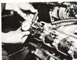
MEASURING THE VALVE CLEARANCE
