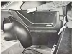
REMOVING THE SIDE TRIM, AT THE REAR SEAT, SAAB 99 WAGONBACK
