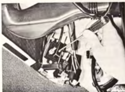
REMOVING THE COVER OF THE COUNTER
