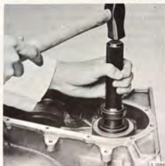
INSTALLING THE BEARING IN THE TORQUE CONVERTER HOUSING
