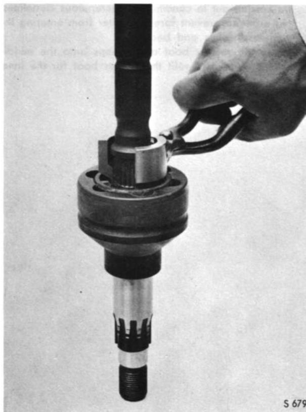
INSTALLATION OF INNER DRIVE SHAFT
