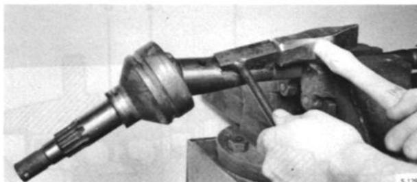
REMOVAL OF INNER DRIVE SHAFT FROM OUTER UNIVERSAL JOINT WITH TOOL 784202
