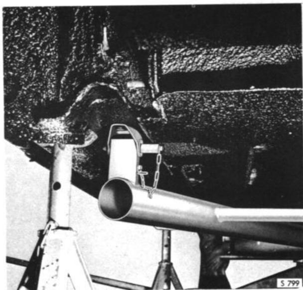
FITTING TOOL No. 784077 IN THE BRACKETS FOR THE REAR-AXLE SIDE LINKS
