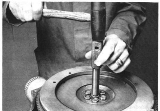
**REPLACEMENT OF DISC-SHAFT BUSHING**
