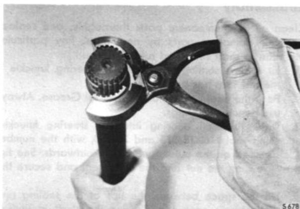
PLACING THE LOCK RING IN TOOL 784161
