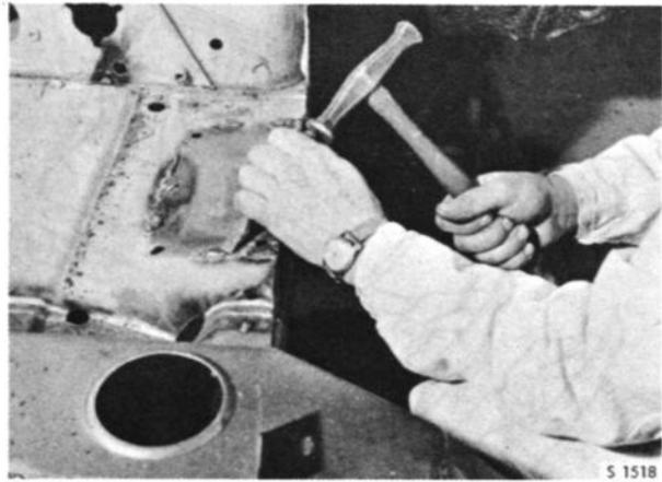
REMOVING TACK-WELDED BODY PANELS
