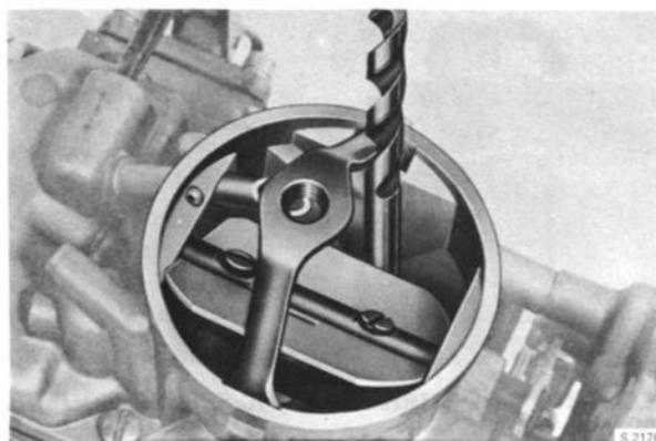
CHECKING CHOKE PLATE OPENING
