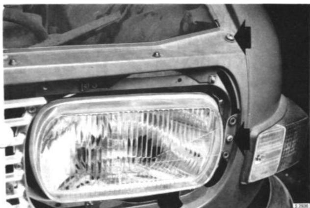
**REMOVAL OF SCREWS, FRONT PANEL**
