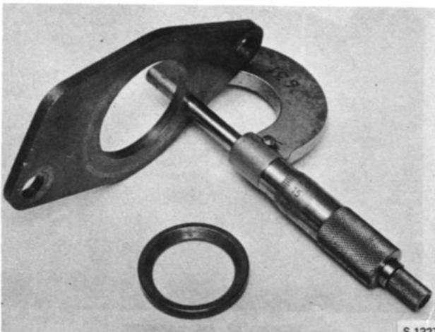
MEASUREMENT OF THRUST PLATE
