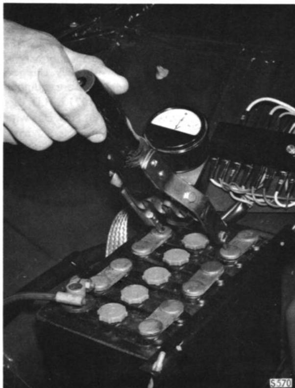
CHECKING THE BATTERY WITH A CELL TESTER
