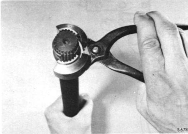
**PLACING OF LOCK RING IN TOOL 784161**
