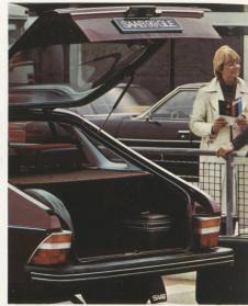
the ground to the rear floor is only 20.9 in. On other cars, it is often as much as 24 – 28 in. When loading heavy objects, the rubber-covered rear bumper can be used as a support. The back door extends from the edge of the roof right down to the bumper.
