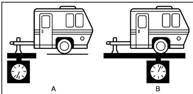
The trailer tongue weight (A) should be 10 percent to 15 percent of the total loaded trailer weight, up to a maximum of 400 lbs (181 kg) with a weight carrying hitch. The trailer tongue weight (A) should be 10 to 15 percent of the total loaded trailer weight, up to a maximum of 750 lbs (340 kg) with a weight distributing hitch.
