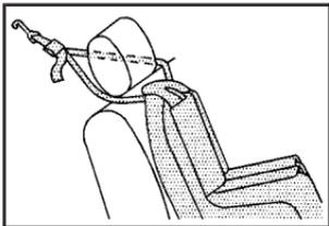
Fold down the head restraint and route the dual tether around the head restraint. See *Rear Seat Operation* on page 1-6.
