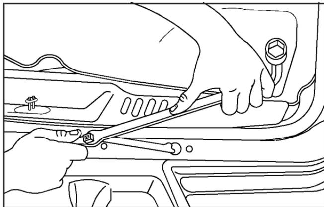
12. Turn the wheel wrench counterclockwise to lower the spare the rest of the way.
