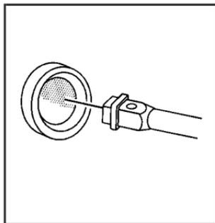
3. Insert the socket end of the extension (C) on a 45 degree angle downward into the hoist drive shaft hole. It is exposed when the rear gate is open and is just above the rear bumper.
