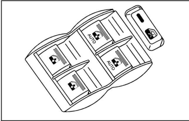
The controls for the power windows are located on the armrest on each of the side doors. With power windows, the switches operate the windows when the ignition is in RUN, ACCESSORY or when Retained Accessory Power (RAP) is active. See *Retained Accessory Power (RAP)* on page 2-21. The driver's door also has a switch for each of the passenger's windows.
