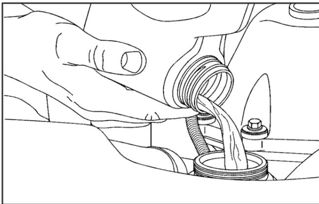
3. Fill the radiator with the proper DEX-COOL® coolant mixture, up to the base of the filler neck. See *Engine Coolant* on page 5-24 for more information about the proper coolant mixture.
