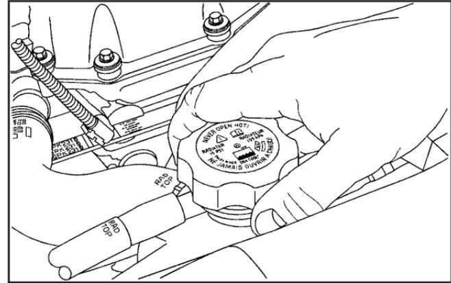
1. You can remove the radiator pressure cap when the cooling system, including the radiator pressure cap and upper radiator hose, is no longer hot. Turn the pressure cap slowly counterclockwise about one full turn. If you hear a hiss, wait for that to stop. A hiss means there is still some pressure left.
