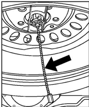
1. Check under the vehicle to see if the cable is visible. If it is not visible, proceed to Step 6.
