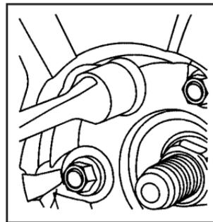
1. Using the wheel wrench, loosen all the wheel nuts. Do not remove them yet.
