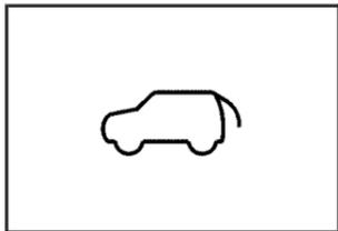
If this light comes on, your liftgate or liftglass is not completely shut.
