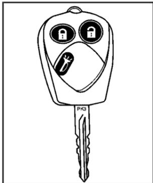
**🔓 (Unlock):** Press the unlock button to automatically unlock the driver's door. The parking lamps may flash and the interior lights will go on. Press the unlock button again and all remaining doors will unlock.
