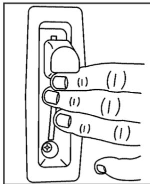
The rear seatback levers are located on the outboard side of each rear seatback.
