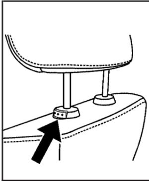
Pull the head restraint up to raise it. Press the release button, located at the base of the head restraint, and push the head restraint down to lower it.
