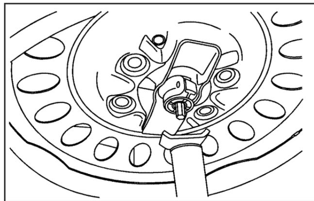
2. If visible, first try to tighten the cable by turning the wheel wrench clockwise until you hear two clicks or feel it skip twice. You cannot overtighten the cable.
