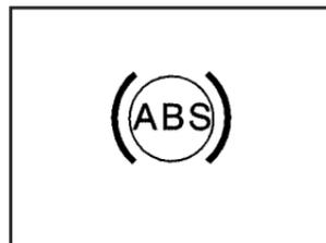
With the anti-lock brake system, this light will come on when you start your engine and may stay on for several seconds, that is normal. A chime may also sound when the light comes on.
