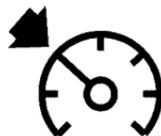
Some vehicles have a cruise light on the instrument panel cluster that will come on when the cruise control is engaged.
