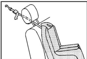
Fold down the head restraint and route the single tether under the head restraint and in between the head restraint posts. See *Rear Seat Operation* on page 1-6.
