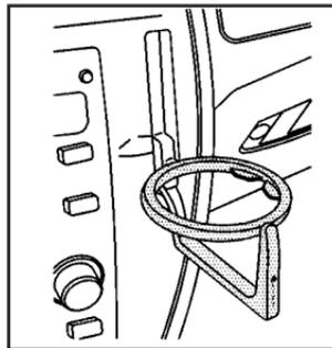
Your vehicle is equipped with a cupholder on the instrument panel next to the radio. To open the cupholder, push once on the arm and the cupholder will move into position for use. To close the cupholder, lift the arm up towards the instrument panel.
