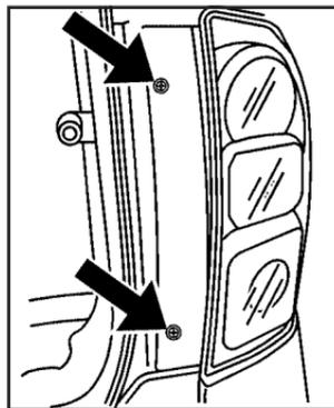
2. Remove the screws from the taillamp assembly.
