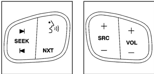
Some audio controls can be adjusted at the steering wheel. They include the following:
