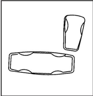
The power seat controls are located on the outboard side of the front seat cushions. The horizontal control adjusts the seat cushion and the vertical control adjusts the seatback.
