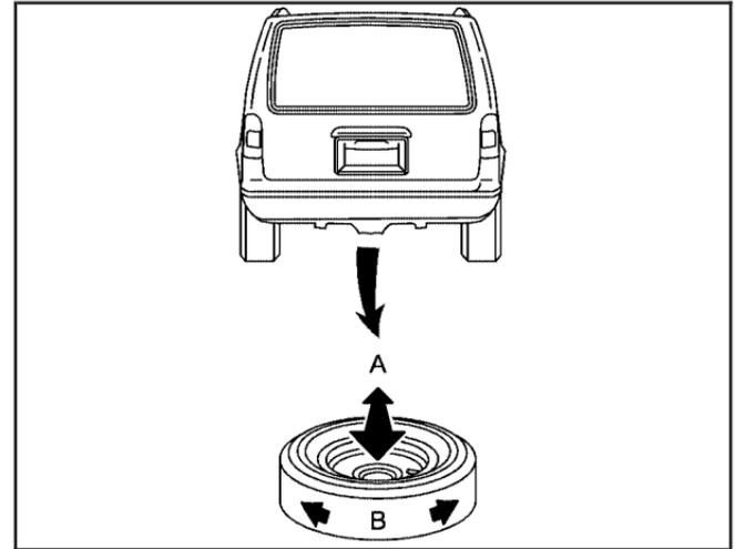
6. Make sure the tire is stored securely. Push, pull (A), and then try to turn (B) the tire. If the tire moves, use the wheel wrench and socket end of the extension to tighten the cable.
