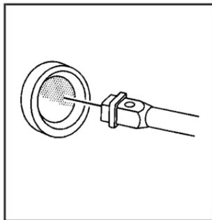
11. If the spare tire is hanging from the cable, insert the socket end of the extension connected to the wheel wrench into the hoist shaft hole just above the rear bumper on a 45 degree angle downward.
