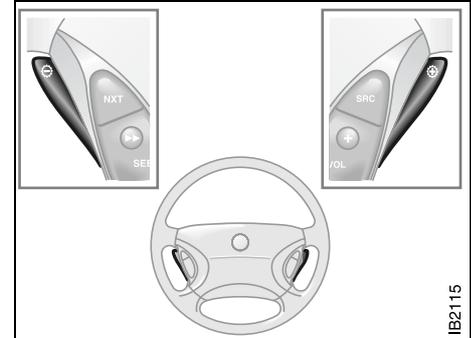
*Paddles on the steering wheel for changing gear manually*
