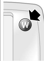
The Winter mode facilitates pulling away and driving on icy roads. Third gear is selected automatically for pulling away to reduce wheelspin. Winter mode can be selected when the engine is running by pressing the "W" button on the selector-lever surround. It cannot be selected when the selector lever is in position M or L. Note: It is still possible to use kick-down in the Winter mode, in which case a change-down to 1st or 2nd will take place.
