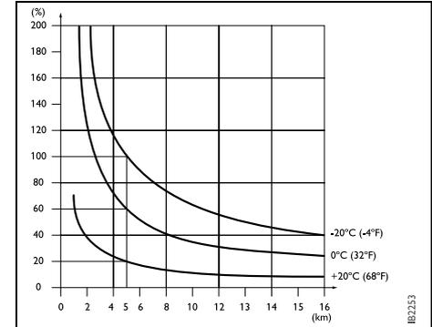
*Percentage increase in fuel consumption of engine starting from cold compared to engine at normal temperature.*
