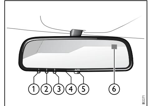
*Buttons for garage opener, autodimming and compass*
