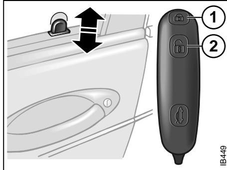
*Locking/unlocking by remote control. Illustration shows the separate remote*
