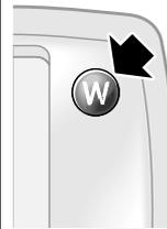
The Winter mode facilitates pulling away and driving on icy roads. Third gear is selected automatically for pulling away to reduce wheelspin. Winter mode can be selected when the engine is running by pressing the "W" button on the selector-lever surround. It cannot be selected when the selector lever is in position 2 or 1.
