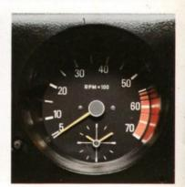
Full instrumentation in the EMS includes a tachometer and clock. All instruments have black borders to eliminate annoying reflections.
